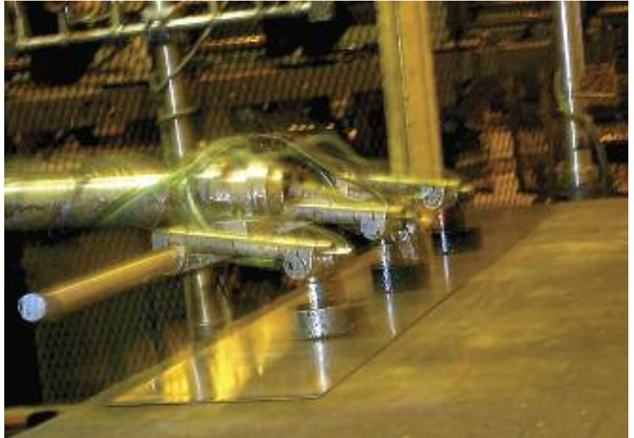
Tower's press-setup crews can easily customize end effectors with a combination of suction cups and retrofittable low-profile magnets, thanks to its use of these 3-in.-dia. Transporter magnets that thread onto the typical 3/8-in. NPT vacuum-cup tooling.
