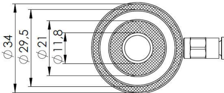
Figure 1. The gripping surface and magnetic poles of MAP-6.
