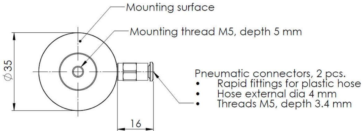
Figure 6. Mounting dimensions of MAP-6. Top view.
