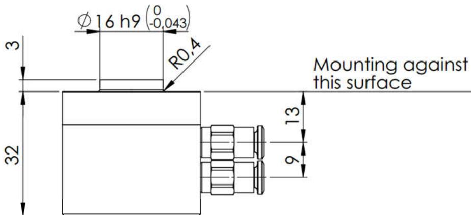
Figure 4. Mounting dimensions of MAP-6
